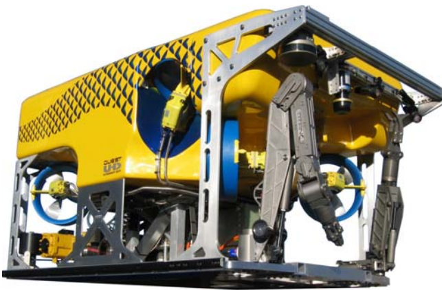
Figure 22 – Remotely Operated Vehicle (ROV) – ROV making electrical connection (courtesy of Schilling Robotics - www.ssaalliance.com )
