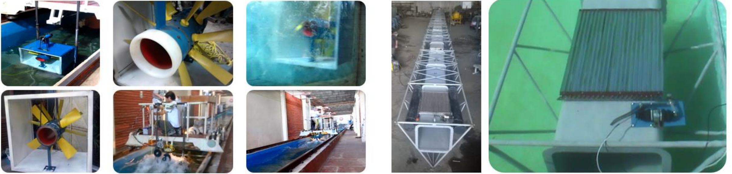
Figure 3.2 "Etymol 1:5 Scale Model Wave Power Plant", "Power Take Off" testing, water tank trial of the "Axial Turbine", "WEC Vessel" testing and "Damper Gates for Seawater Entrance" testing. In the photography testing, the "Damper Gates" position is closed.
