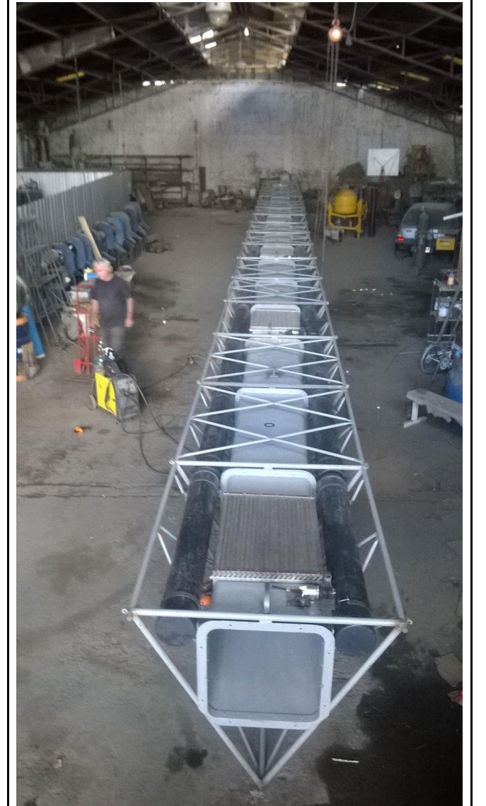
Figure 5.1 "Etymol 1:5 Scale Model Wave Power Plant".
