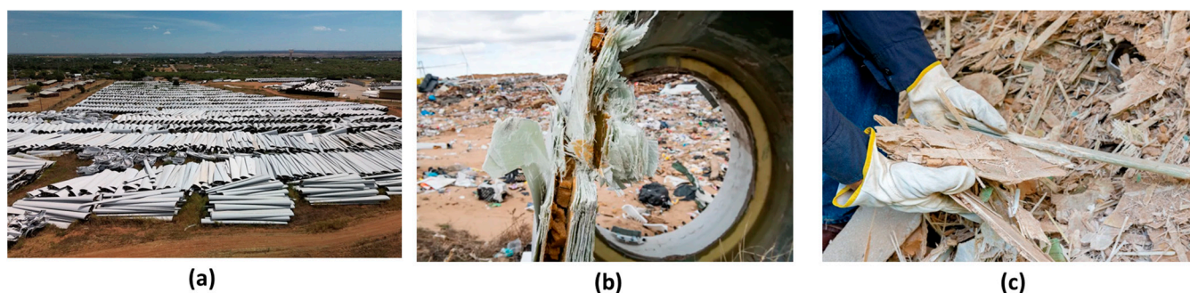
Figure 1. Pictures of decommissioned blades (a) Discarded wind turbine blades in west Texas (photo by Eli Rosen) [6], (b) blade in Colorado landfills (photo by Andy Colwell) [7], and (c) shredded pieces of blades for recycling (photo from Veolia) [8].
