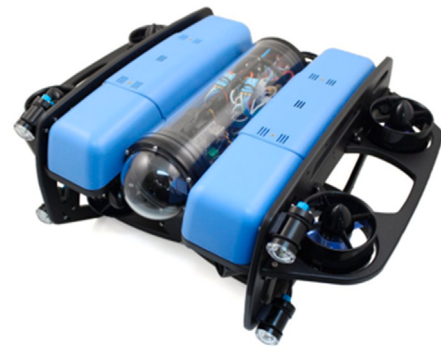
Fig. 2. BlueROV2 UUV (BlueRobotics, 2023).
